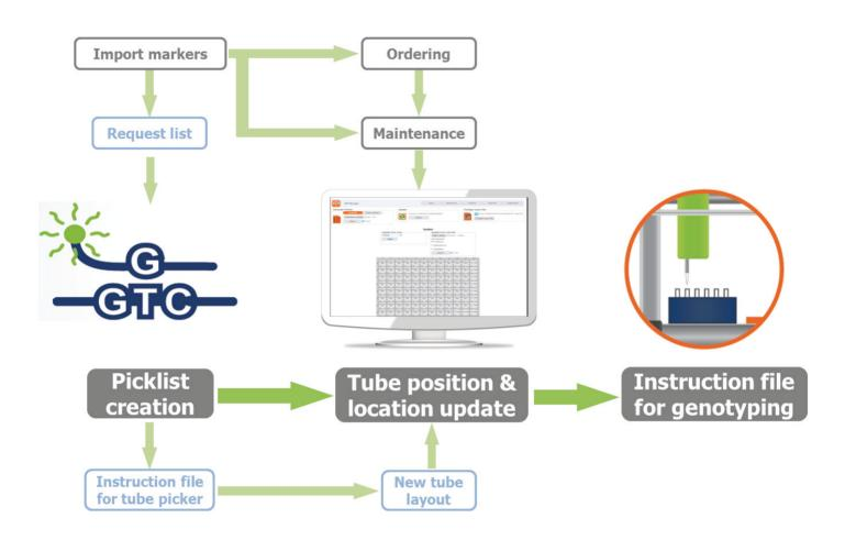
Combined with LabCollector **Samples** and **Documents** modules, the SNP Manager add-on allows users to manage tubes and plates containing markers: storage location, stock quantity, status (available, ordered...) and suppliers ordering with a few clicks.
